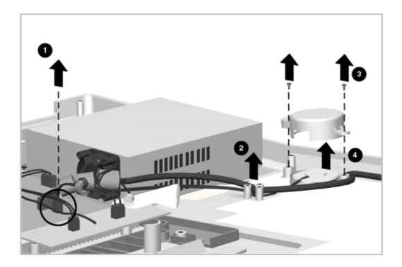
Figure 6-28. Removing the Speaker Assembly
